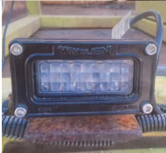
Second Generation Lights. Brighter but more focused on the lane directly behind the unit.
