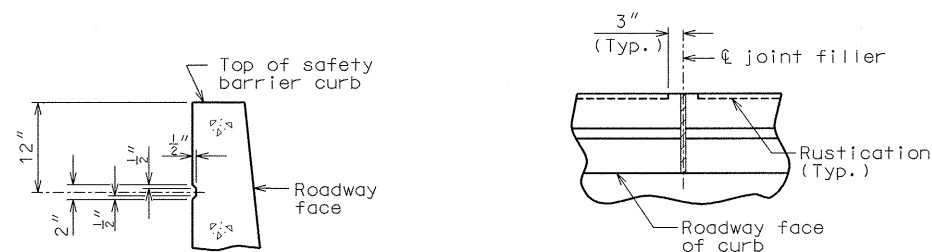
PART SECTION SHOWING RUSTICATION DETAILS
