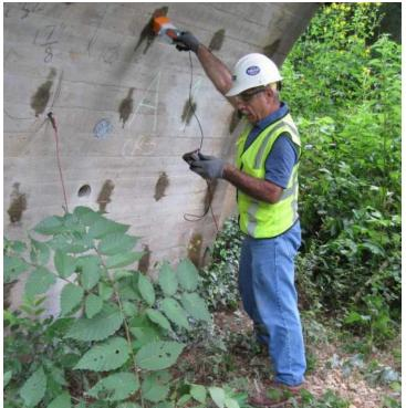
Photo 7: Half Cell Potential Testing
