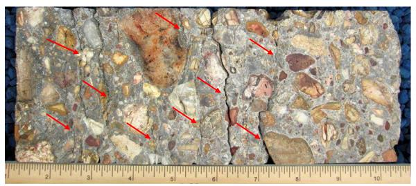
Figure 2: Photograph showing the cracks in Core CR-1. The outer surface is to the left. Scale in inches.
