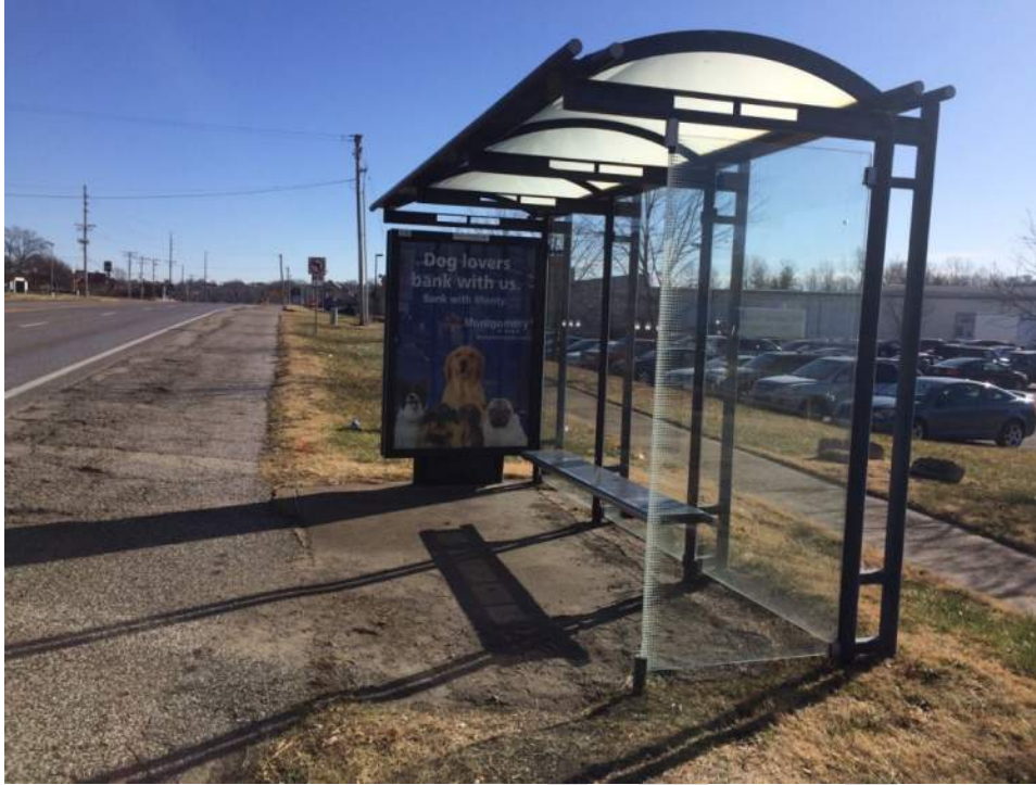
Bus Shelter along shoulder. Sidewalk behind shelter but not connected up to shoulder.
