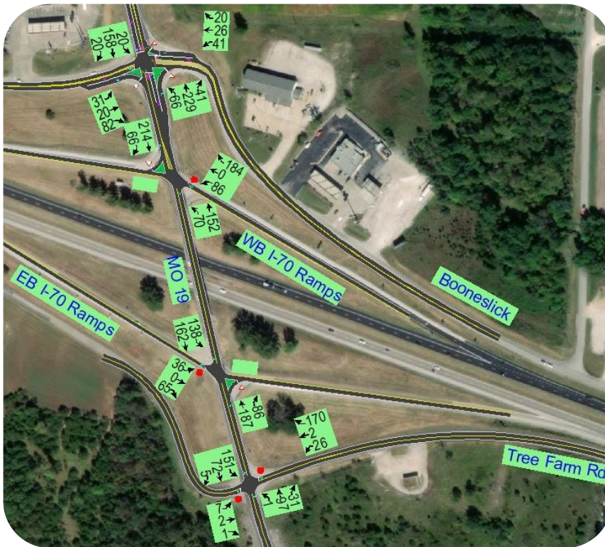
Figure 5: Projected Construction Year (2021) AM Peak Hour Volumes
