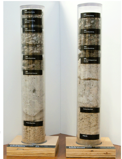
These core samples of I-70 pavement in Saline and Boone Counties show just how much the pavement beneath the surface has deteriorated under years and years of growing traffic.
