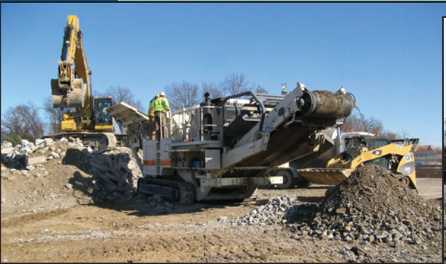
ABOVE: Demolition begins on the eight-month reconstruction of the Hanley Road bridge over I-64. For an illustration of the Hanley detour route, see page four. BELOW LEFT: Concrete from demolished bridges and pavement is crushed and turned into fill material for new roadbed near Laclede Station Road. BELOW MIDDLE & RIGHT: Demolition of the I-64 bridge over Claytonia Terrace will close that street for as long as 90 days. A total of nine structures will be rebuilt on the second half of the project.
