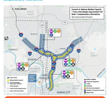
Includes an additional lane in each direction for the limits shown, plus rebuilding the focus interchanges plus complementary alternatives.
