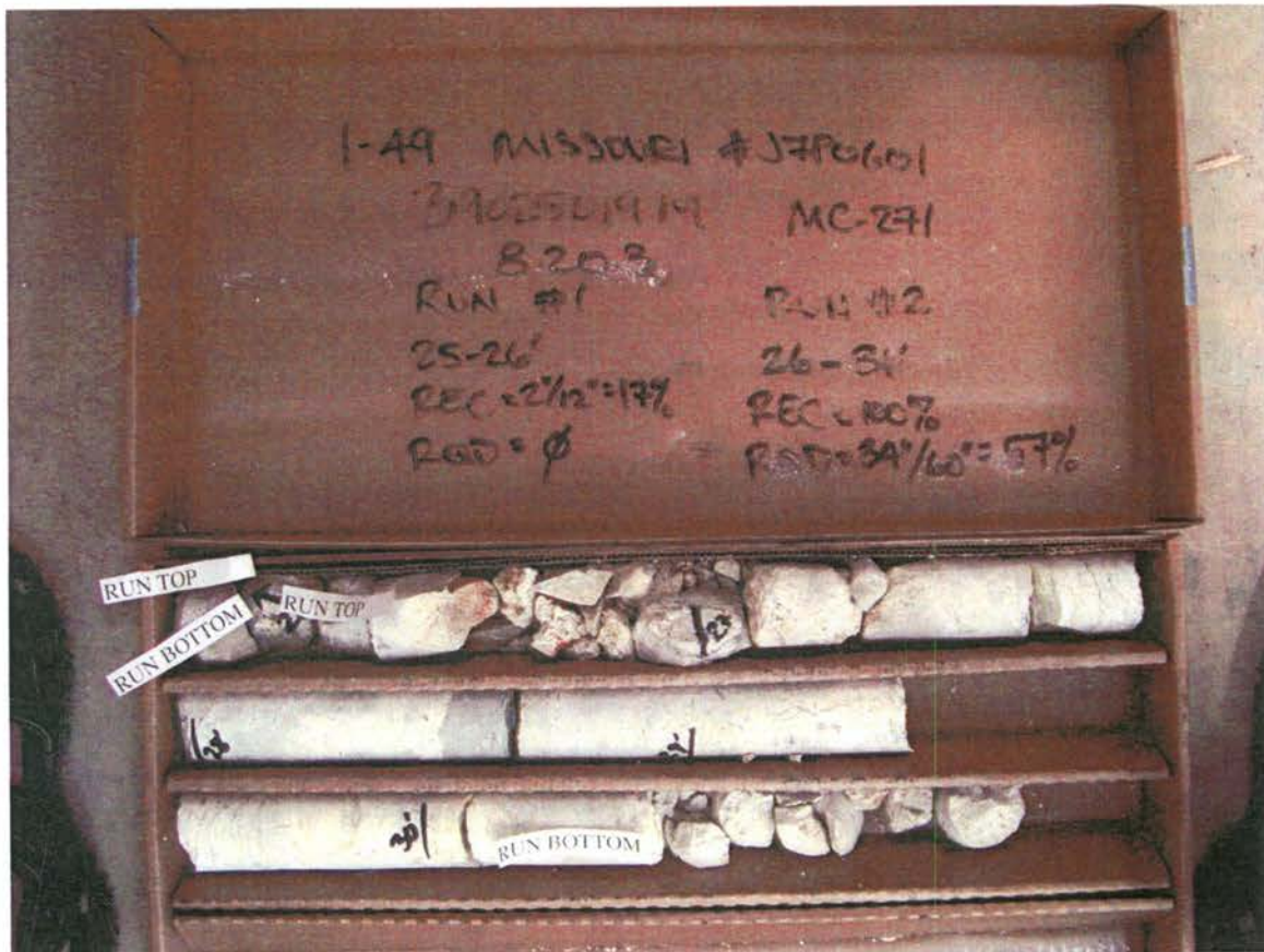
I 49 Missouri Missouri J7P0601 Boring No. MC 271 Run No. 1 25.0 Feet to 26.0 Feet Run No. 2 26.0 Feet to 31.0 Feet
