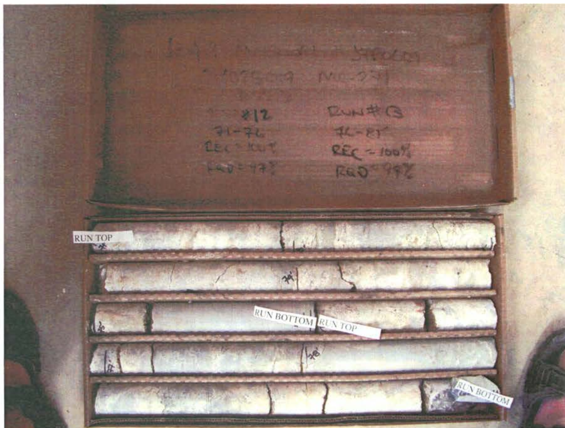
I 49 Missouri Missouri J7P0601 Boring No. MC 271 Run No. 12 71.0 Feet to 76.0 Feet Run No. 13 76.0 Feet to 81.0 Feet
