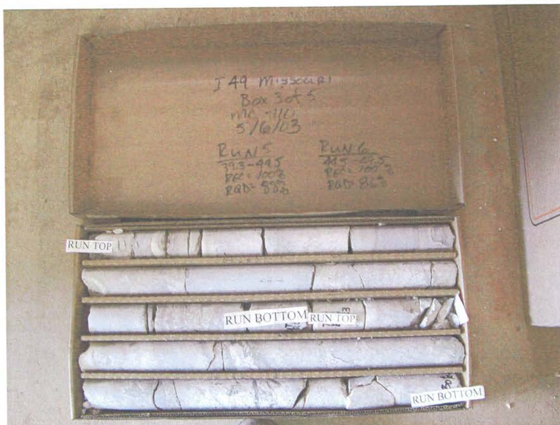
I 49 Missouri Missouri J7P0601 Boring MC-110 Run No. 5 39.5 Feet to 44.5 Feet Run No. 6 44.5 Feet to 49.5 Feet
