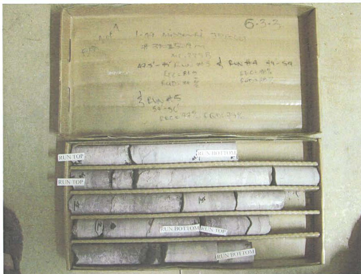
I 49 Missouri Missouri J7P0601 Boring No. MC 229B Run No. 3 47.5 Feet to 49.0 Feet Run No. 4 49.0 Feet to 54.0 Feet Run No. 5 54.0 Feet to 56.0 Feet
