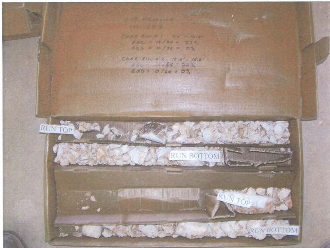
I 49 Missouri Missouri J7P0601 Boring MC-253 Run No. 1 7.0 Feet to 10.0 Feet Run No. 2 10.0 Feet to 15.0 Feet
