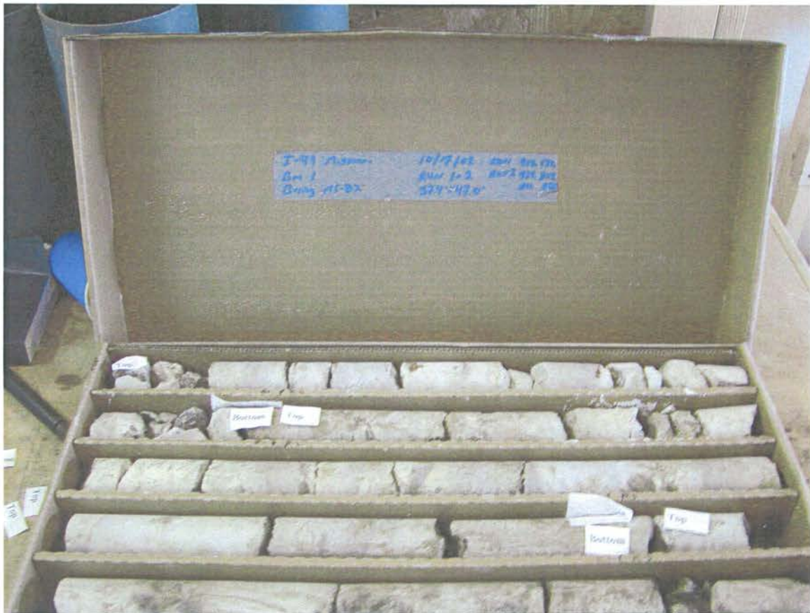
I 49 Missouri Missouri J7P0601 Boring MC-82 Run No. 1 37.4 Feet to 40.0 Feet Run No. 2 40.0 Feet to 45.0 Feet Run No. 3 (partial) 45.0 Feet to 50.0 Feet
