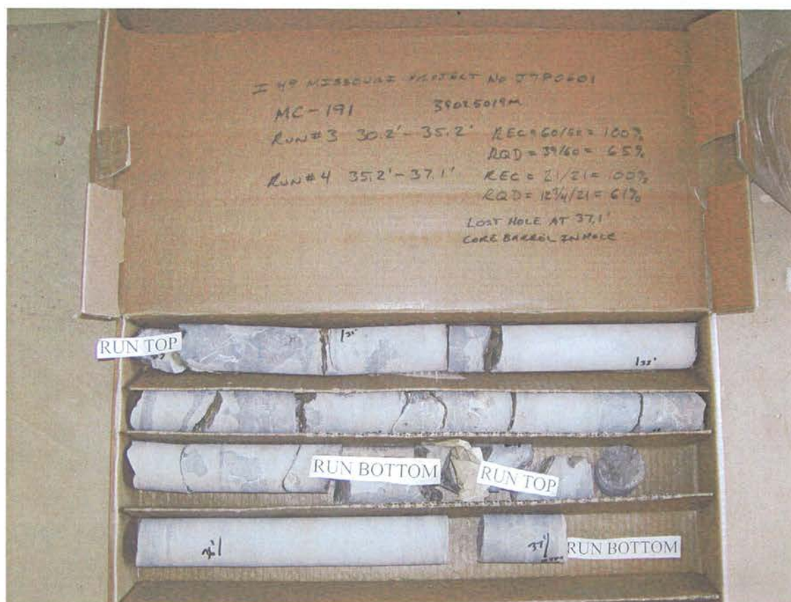
I 49 Missouri Missouri J7P0601 Boring MC-191 Run No. 3 30.2 Feet to 35.2 Feet Run No. 4 35.2 Feet to 37.1 Feet
