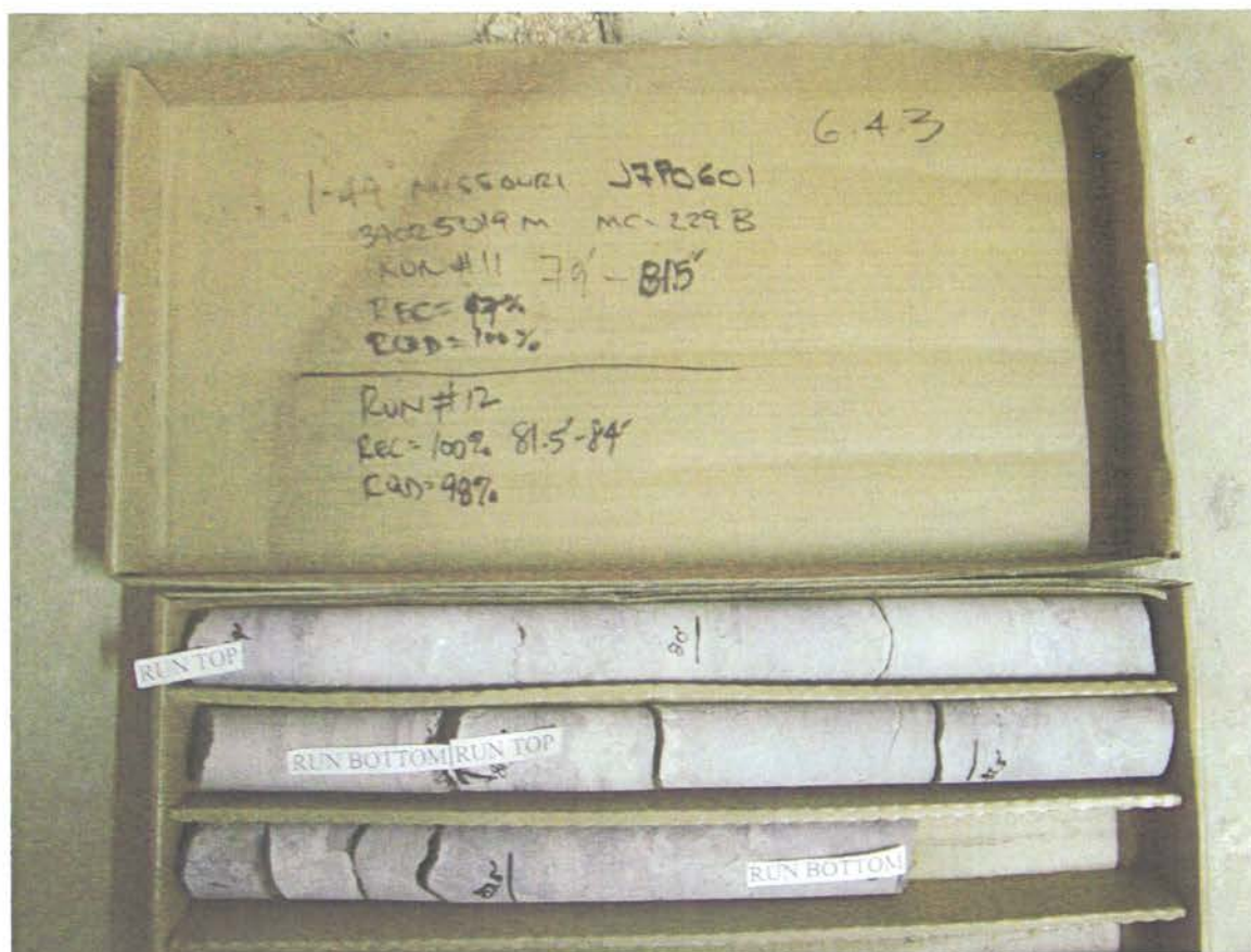
I 49 Missouri Missouri J7P0601 Boring No. MC 229B Run No. 11 79.0 Feet to 81.5 Feet Run No. 12 81.5 Feet to 84.0 Feet
