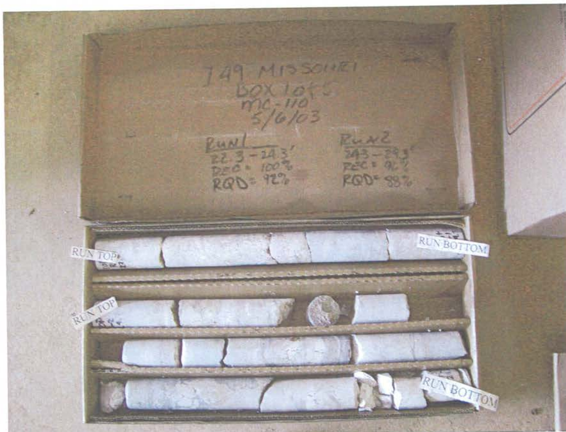
I 49 Missouri Missouri J7P0601 Boring MC-110 Run No. 1 22.3 Feet to 24.3 Feet Run No. 2 24.3 Feet to 29.3 Feet
