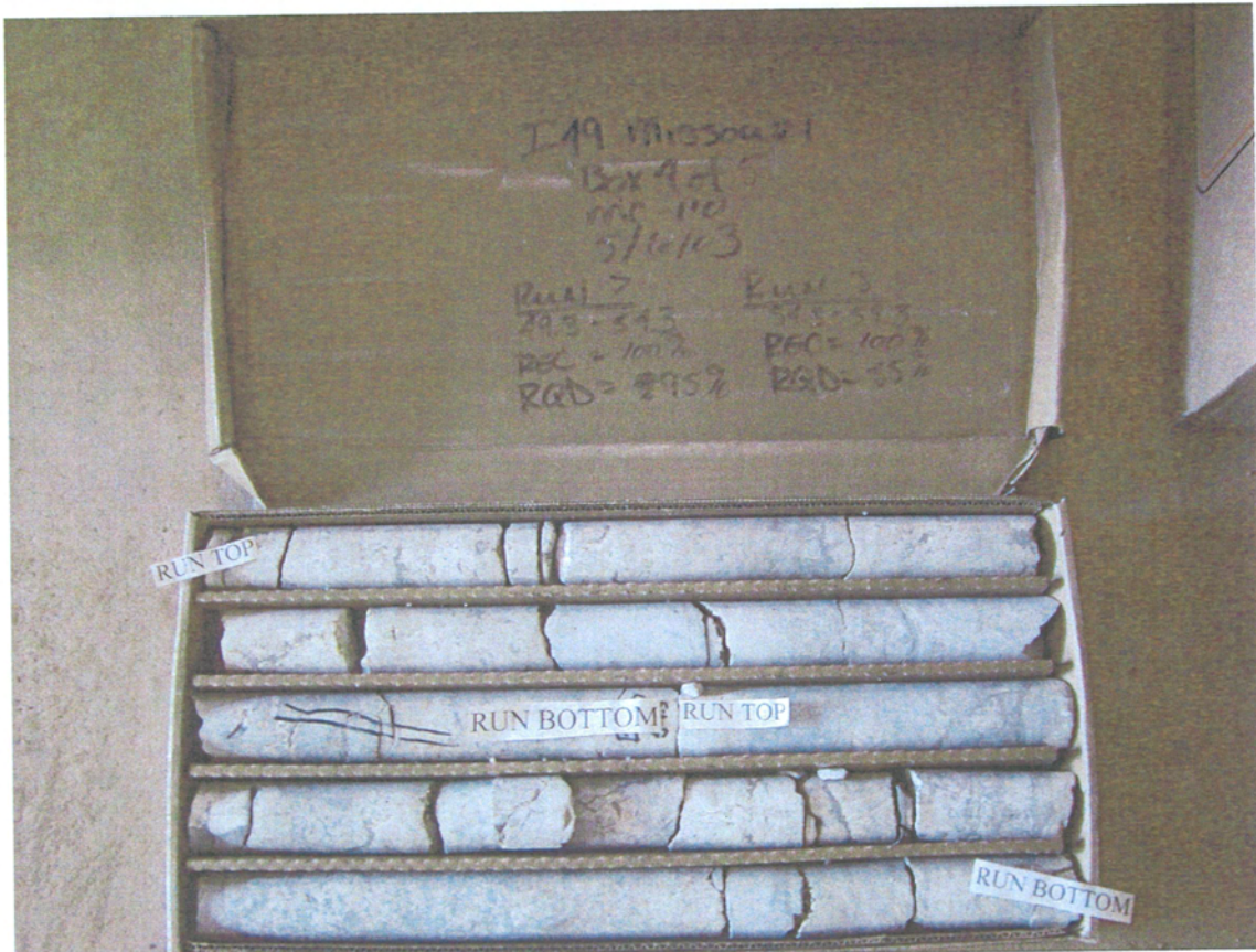
I 49 Missouri Missouri J7P0601 Boring MC-110 Run No. 7 49.3 Feet to 54.3 Feet Run No. 8 54.3 Feet to 59.3 Feet
