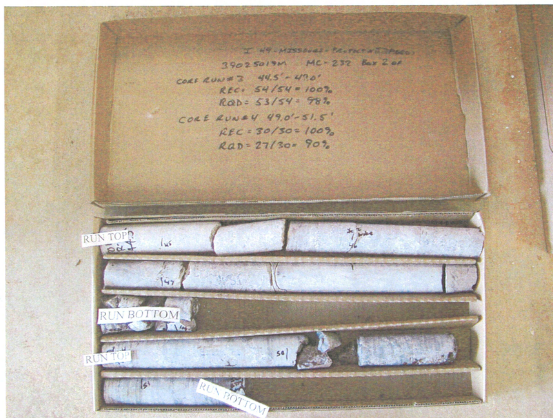
I 49 Missouri Missouri J7P0601 Boring MC-229 Run No. 3 44.5 Feet to 49.0 Feet Run No. 4 49.0 Feet to 51.5 Feet
