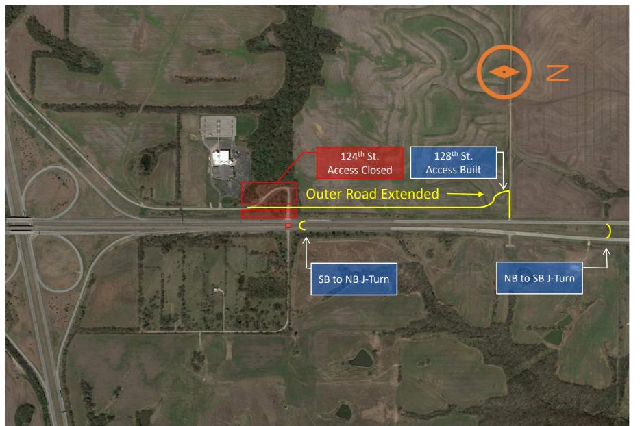
Construct a right-in/right-out access on US-169 at N.W. 128<sup>th</sup> Street
