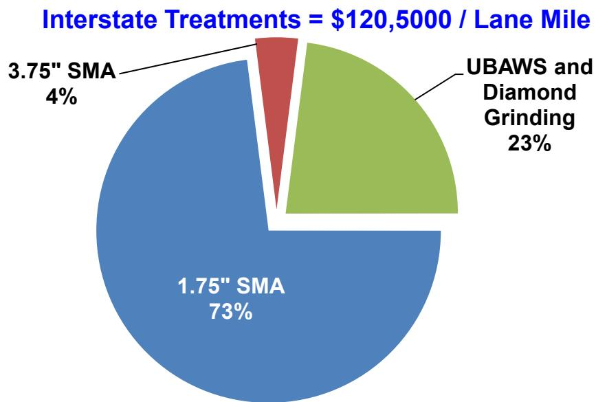
Using the Asset Management System described in Chapter 2, MoDOT can determine the life cycle for assets. For example, the treatments assumed for interstates are expected to keep the pavement in good condition for 8 years. The following chart shows how interstate treatment data is used to confirm pavements remain in good condition for an average of 8 years.
