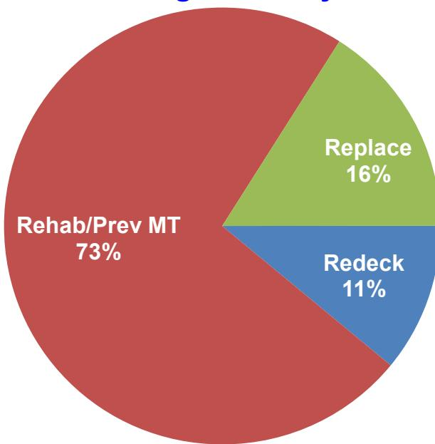
The bridge work represented above varies in price per bridge and type of work being performed. The overall costs are as follows: Replacements - \$279/sf; Redeck - \$89/sf; Rehab/Preventive Maintenance \$35/sf and represents approximately 80 bridges each year getting work performed on them. This work is needed to keep each bridge in a state of good repair on the NHS, with much more work needed on non-NHS bridges to keep MoDOT's entire bridge network in a state of good repair.
