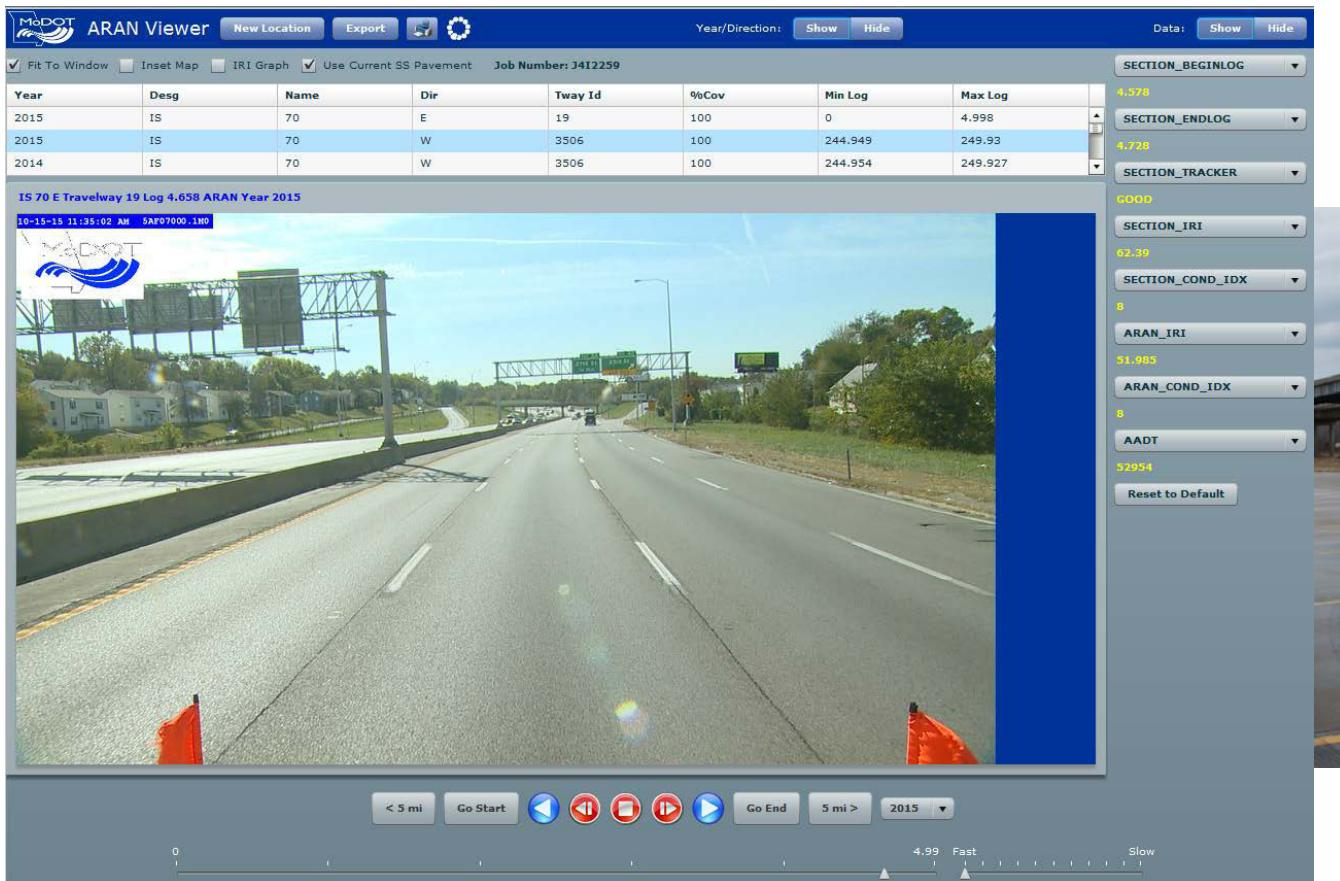
TMS applications (as shown on the following page) capture and store all historical pavement data. MoDOT pavement experts then query this historical information and analyze the data using spreadsheets to determine how well the pavement has performed and to establish future pavement deterioration rates for pavement sections. TMS is MoDOT's Pavement Management System (PMS) as it has multiple applications that aid in establishing the deterioration rate of pavements.
