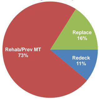
The bridge work represented above varies in price per bridge and type of work being performed. The overall costs are as follows: Replacements - \$279/sf; Redeck - \$89/sf; Rehab/Preventive Maintenance \$35/sf and represents approximately 80 bridges each year getting work performed on them. This work is needed to keep each bridge in a state of good repair on the NHS, with much more worked needed on non-NHS bridges to keep MoDOT's entire bridge network in a state of good repair.
