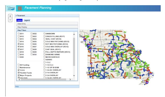
MoDOT has historically analyzed pavement data and tracked progress of pavement by smoothness. Smoothness is measured by international roughness index (IRI), the lower the IRI, the smoother the road. Shown below are the MoDOT rating categories for NHS pavements for smoothness:
