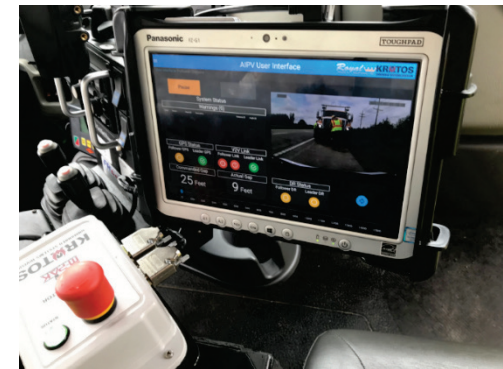
Figure 6. | User Interface in the MoDOT Autonomous TMA Pilot
