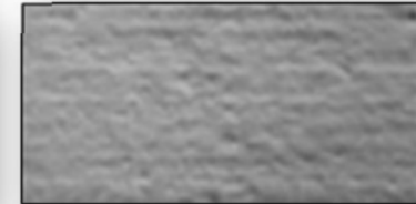
CSP 4 (light scarification)
