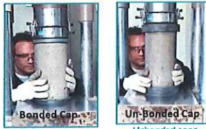
Bonded Cap Sulfur mortar cap AASHTO T231
