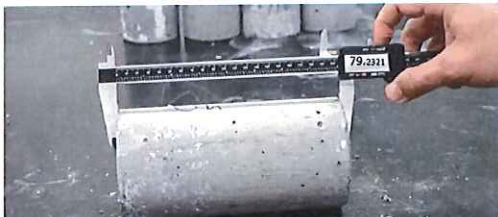
Measure diameter and length of cylinder
