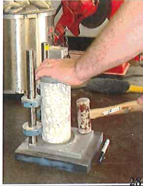
Capping with Sulfur Mortar
