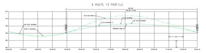
PROPOSED PROFILE VERTICAL CURVE MEETS 60 MPH DESIGN CRITERIA EXISTING PROFILE VERTICAL CURVE MEETS 45 MPH DESIGN CRITERIA
