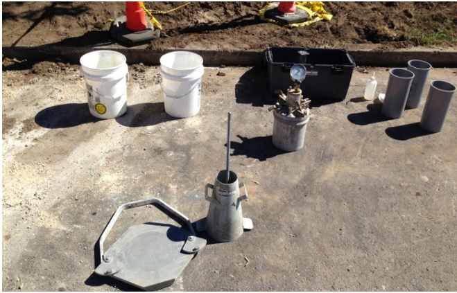
Example of Bartlett & West Humboldt Type B air meter, slump cone, and cylinder molds for concrete materials testing and sampling.
