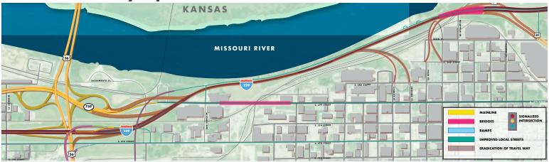
This alternative removes the Interstate classification from Hwy 36 to at least Highland Avenue. In this section, I-229 is decommissioned, the double-decker bridge removed, and a scenic 2-lane parkway is constructed. The 2-lane parkway would be constructed at grade (must comply with floodplain and stormwater drainage requirements) in generally the same location as the existing double-decker bridge between the Burlington Northern Railroad tracks and the Missouri River.
