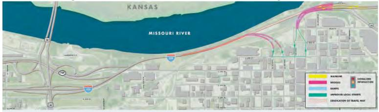
This alternative would remove at least a portion of the Interstate classification between Hey 36 and Hwy 59. I-229 would be decommissioned between the downtown ramps, the double-decker bridge removed, and traffic routed through downtown via reconnection at South 3rd Street. The double-decker bridge would remain south of the Charles Street/ Edmond Street ramps and would require rehabilitation/ maintenance. All of the downtown ramps would stay in their current location.
