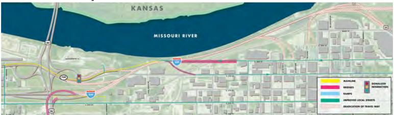
This alternative removes the Interstate classification between Hwy 36 and Hwy 59. In this section, I-229 is decommissioned, the double-decker bridge removed, and nothing constructed in its current location, opening up the riverfront. Traffic is routed through downtown on local collector streets.
