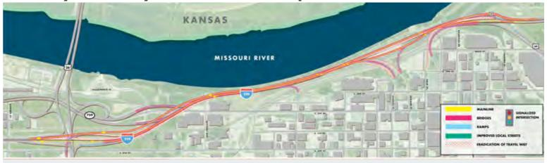
This alternative would leave the Interstate classification through the entire corridor. In this alternative, the double-decker bridge would be removed, and I-229 reconstructed. The Interstate would be constructed with long, one-lane elevated ramps connecting Interstate stubs at both ends of the project.
