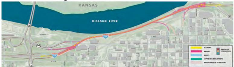
This alternative would repurpose the existing double-decker bridge and maintain an interstate system through the corridor between the Burlington Northern Santa Fe Railroad and the Missouri River. The top deck of the existing double-decker bridge would be removed, and an additional bridge system would be constructed adjacent and level with the lower deck.
