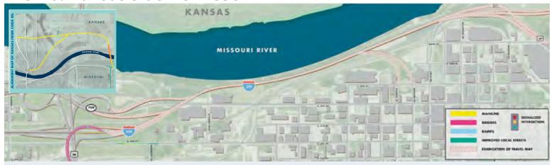
This alternative consists of the relocation of the mainline I-229 corridor from the east side of the Missouri River to the west side of the Missouri River. I-229, near Cook Road, would curve to the west and cross over the Missouri River. The bridge structure would be approximately 2700 feet long and span the Missouri River and its floodway. A new interchange facility would provide connections between Cook Road and I-229.
