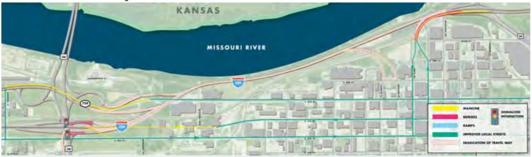
This alternative removes the Interstate classification between Hwy 36 and Hwy 59. In this section, I-229 is decommissioned, the double-decker bridge removed, and nothing constructed in its place, therefore, opening up the riverfront. Traffic is routed through downtown on local collector streets.
