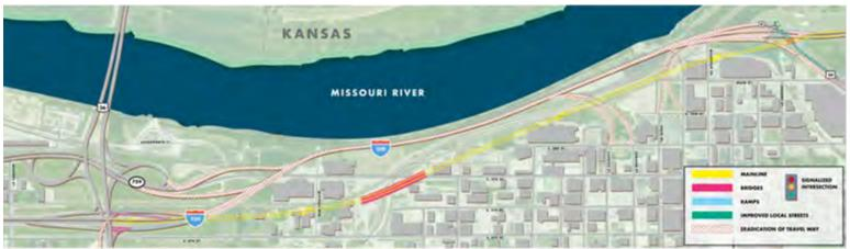
This alternative would leave the Interstate classification through the project area. In this alternative, the double-decker bridge would be removed, and I-229 reconstructed on the east side of the tracks. The Interstate would be generally constructed at grade. A bridge would be required on the north end for a new interchange between Hwy 59 and 1-229.
