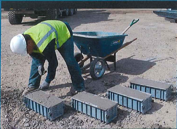
Flexure Beam Test Jig
