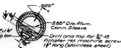
RAIL SPICE OR EXPANSION DETAIL
