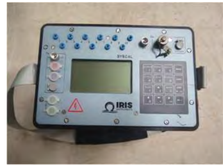
IRIS Syscal Pro-96 10-channel resistivity meter.
