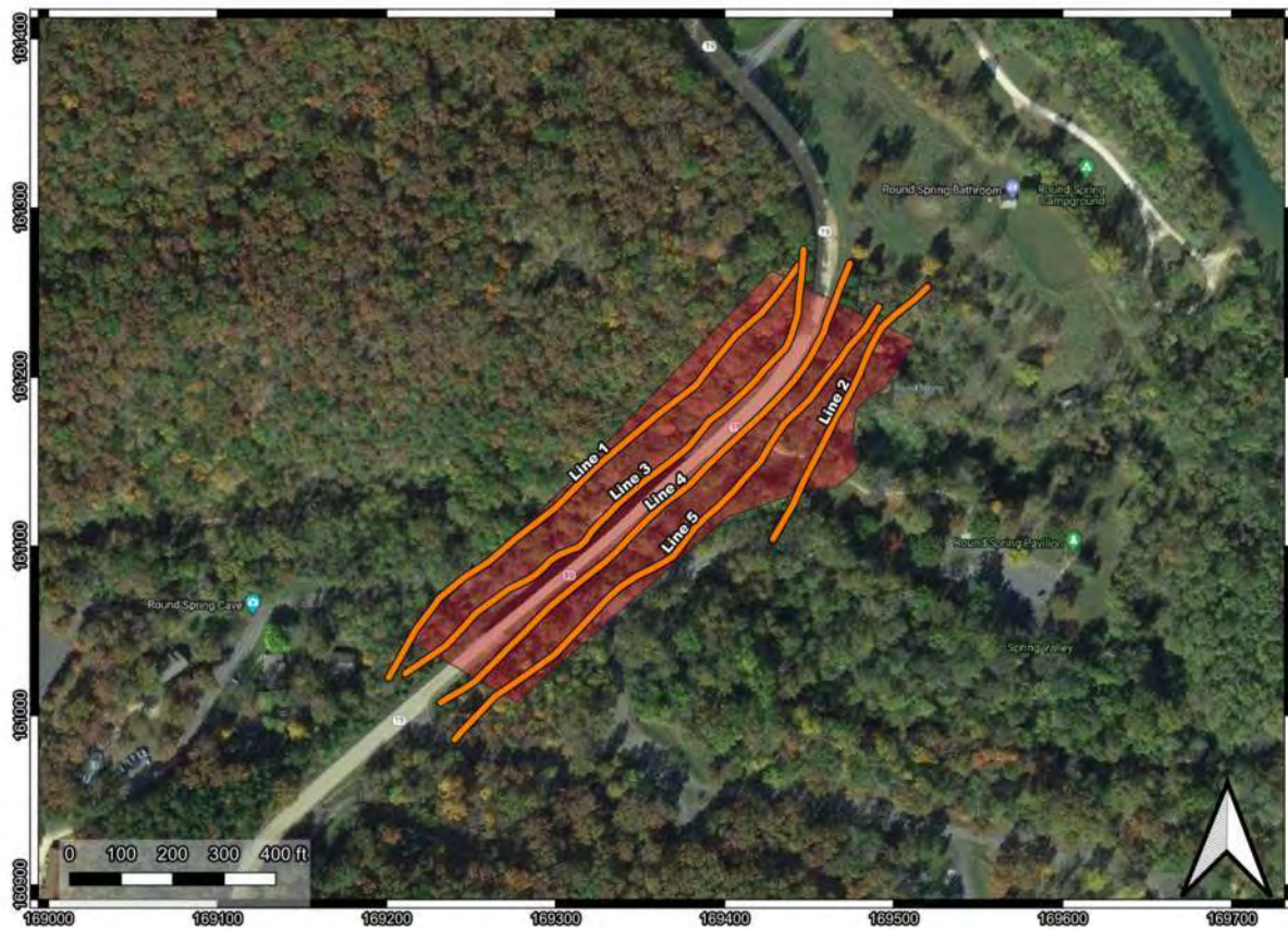
Figure 3: Overview of project area with geophysical (ERT) lines (orange) and approximate area of interest for the investigation (shaded red). The SRT line was collected along the Line 4 profile.
