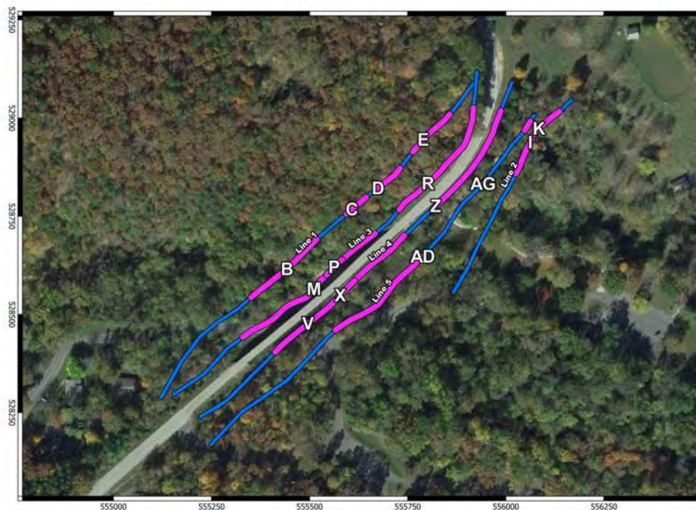
Figure 9: Plan view map of high-resistivity anomaly surface extents. NAD83 State Plane Missouri East US Survey Foot
