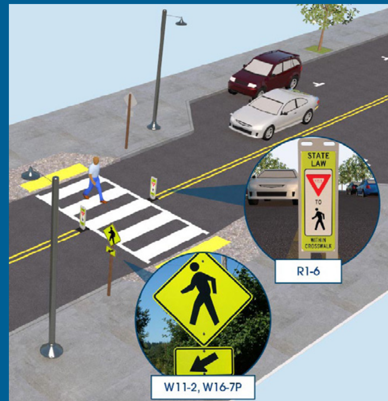
Crosswalk visibility enhancements
