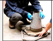
\*\*Complete the test from filling to mold removal in ≤ 2 ½ minutes.
