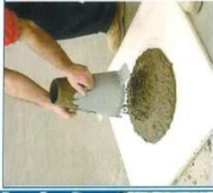
Excessive slump means the concrete has too much water. it's likely to shrink excessively and crack. It will be significantly weaker than properly hydrated concrete.
