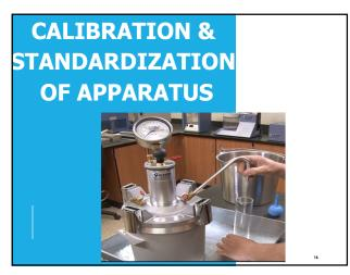
Unless otherwise specified, follow the requirements and intervals for equipment calibrations, standardizations, and checks in AASHTO R 18, and procedures in AASHTO R 61.
