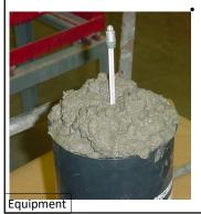
A cylinder mold that is **6**" in diameter is acceptable for the required **3**" coverage around the probe or a bulb of the thermometer or as long as the thermometer bulb is in the center.
