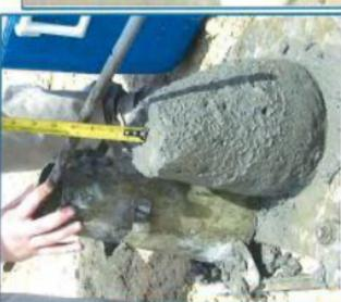
This concrete has about a 3.5 inch Slump. It's wet enough to be poured and vibrated properly yet dry enough that, as it cures, it will reach maximum strength.
