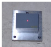
Reading on base plate + 1 inch block + calibration plate (H2)
