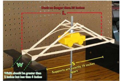
**3.** Bridge width (W) must be 2 inches or greater, but less than 4 inches (for the entire length of the bridge) so that no part of the car touches the
