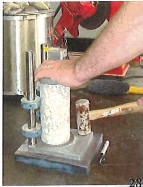
Capping with Sulfur Mortar
