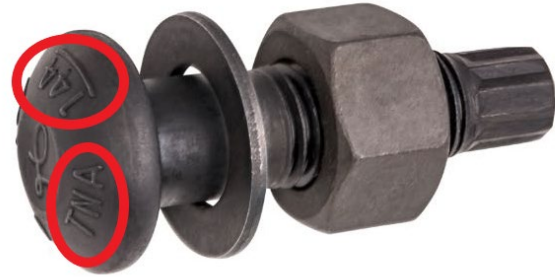
Figure 712.1.5.4.1.3, 144 TNA Fixed Spline Bolt These fixed spline bolts will follow the requirements of ASTM F3148 Grade 144 with TNA (Torque & Angle) also listed on the bolt head.
