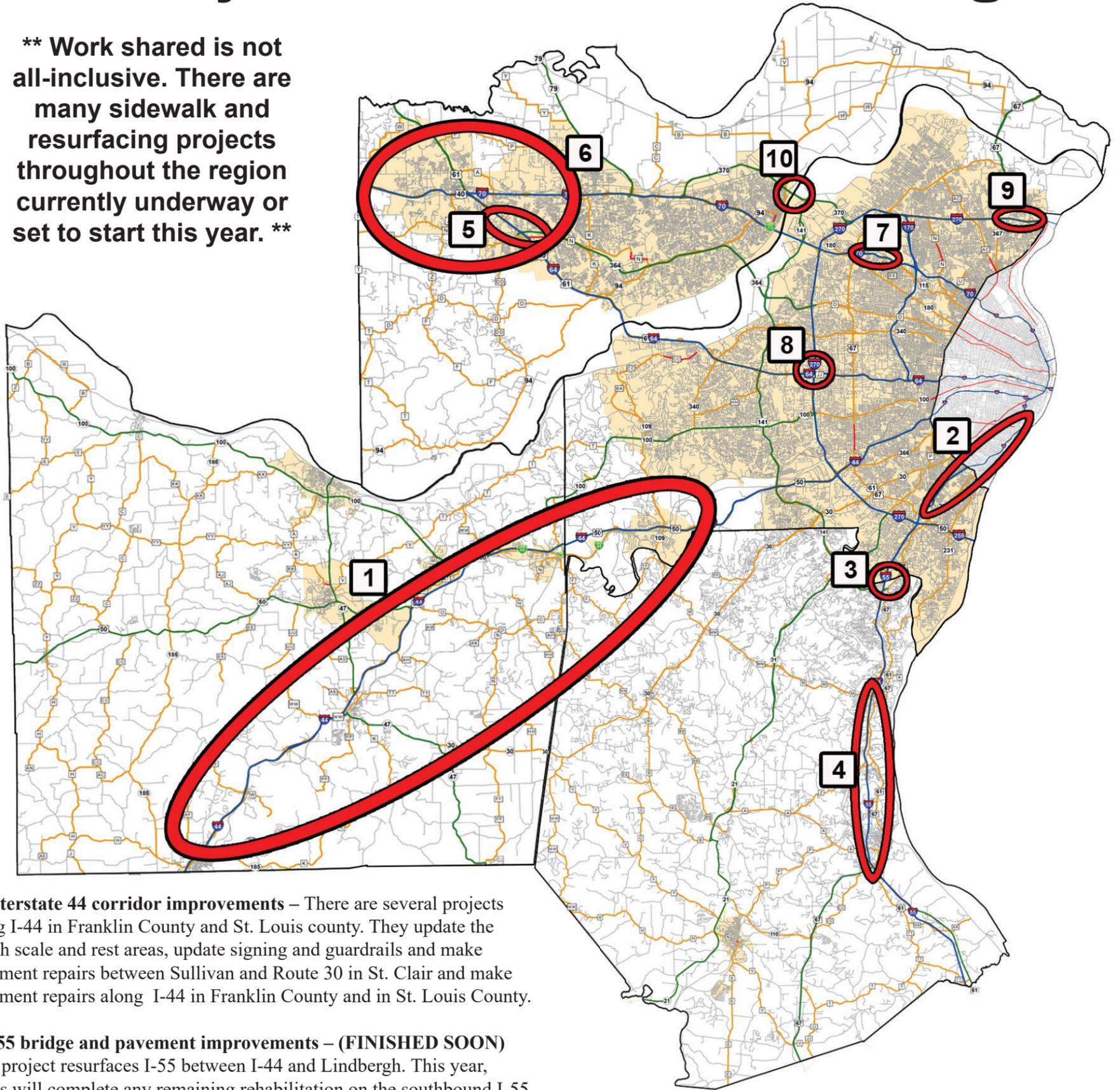
**1. Interstate 44 corridor improvements** – There are several projects along I-44 in Franklin County and St. Louis county. They update the weigh scale and rest areas, update signing and guardrails and make pavement repairs between Sullivan and Route 30 in St. Clair and make pavement repairs along I-44 in Franklin County and in St. Louis County.
