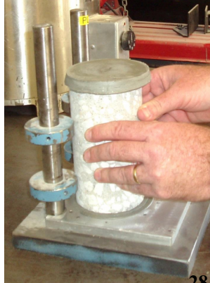
Capping with Sulfur Mortar
