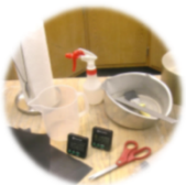
Accessories – timer, knife or scissors, spray bottle of isopropyl alcohol, bucket, syringe, small paint brush, rubber sheets
