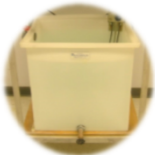
Water Bath – 24 x 18 x 18in. Min., capable of maintaining water temperature of 25±1°C (77±2° F)
