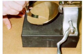
Grooving the soil specimen
