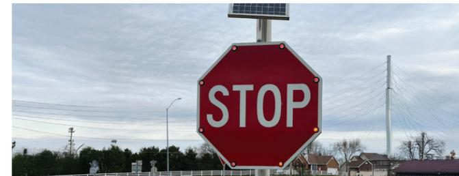
**Stop Sign with Flashing LEDs**
