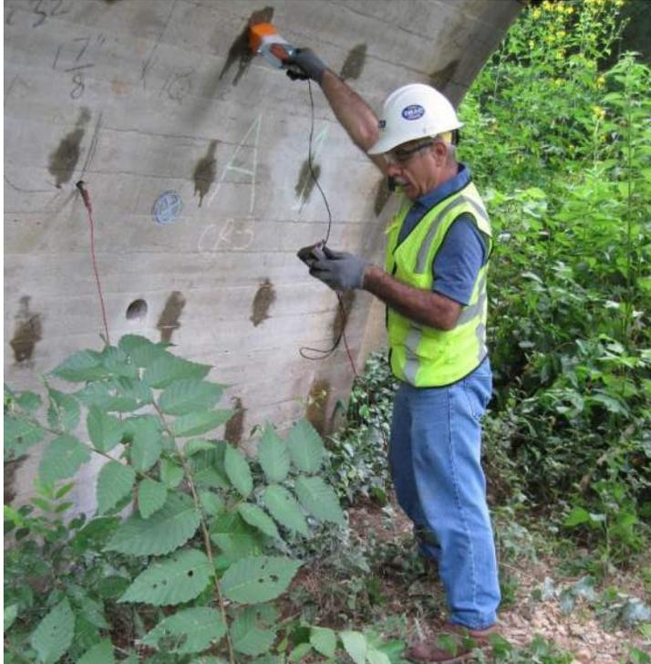
Photo 7: Half Cell Potential Testing
