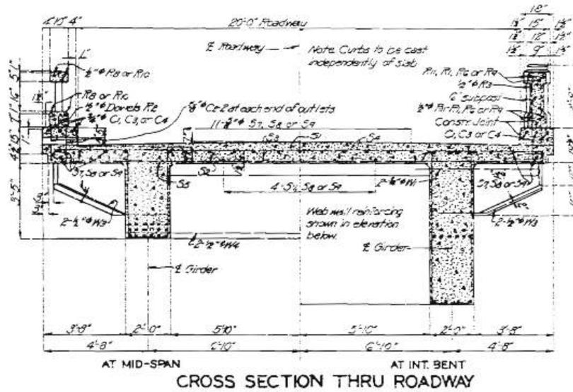
Figure 2-8. Spring Valley Bridge (J0420) Typical Section through Arch Span
