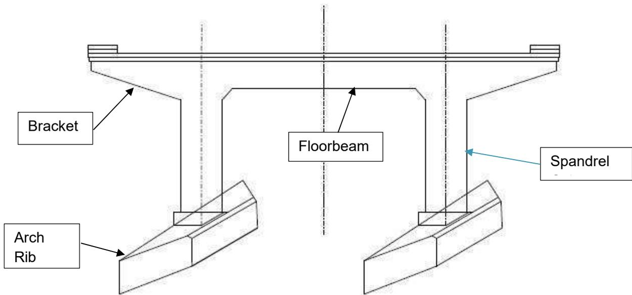
Typical Section Through Arch Span
