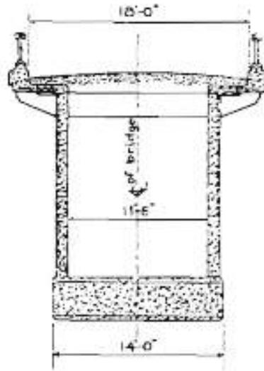
Figure 2-5. Current River Bridge (G0804) Typical Section through Filled Abutment Houses
