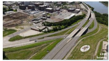
In this alternative the double-decker bridge is removed and replaced with a new four-lane arterial road constructed at-grade (elevated as necessary for compliance with floodplain and stormwater requirements) in generally the same location as the existing double-decker bridge between the railroad tracks and the Missouri River. This alternative would require de-designation of I-229 as interstate.
