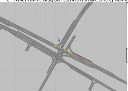
Connecting the two WBR lanes into one larger lane (yellow marking) helps operations at the Valley View signal: the high number of WBR to I-470 can now use a different lane than those headed to either WB US-40 or SB I-470. This can also result in the unique dual SBR being configured more conventionally (blue arrow).
