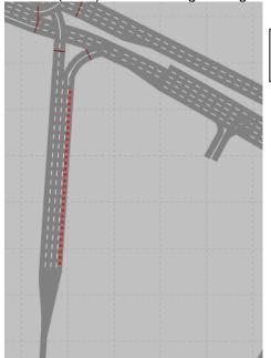
The additional NBR turn lane (red marking) helps reduce the NB queue.
