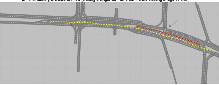
The extension of the Valley View EBL (yellow marking) greatly helps the interchange operations (allows triple SBL at I-470 depicted by blue arrow)
