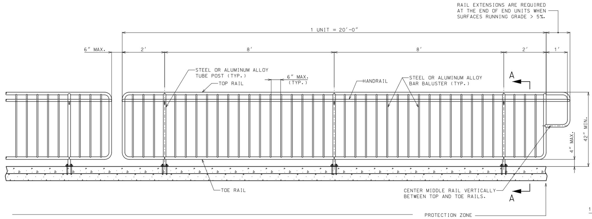
**SIDEWALK SAFETY RAIL WITH BALUSTERS AND HANDRAIL**
