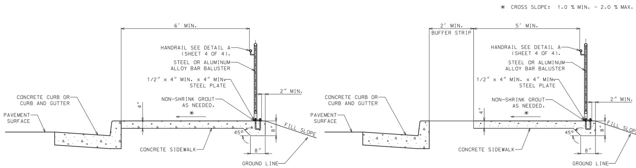
**SIDEWALK WITHOUT BUFFER STRIP (SECTION A-A)**
