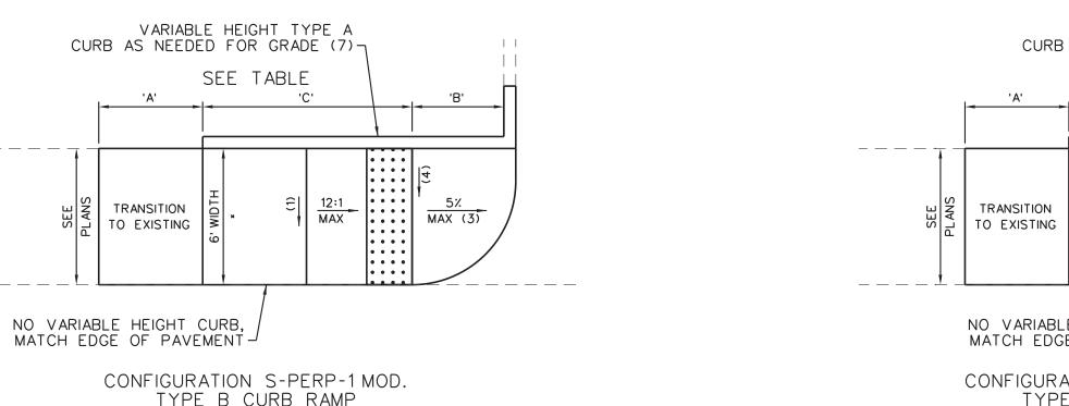
TYPE B CURB RAMP SINGLE PERPENDICULAR, SMALL RADIUS, NO BUFFÉR
