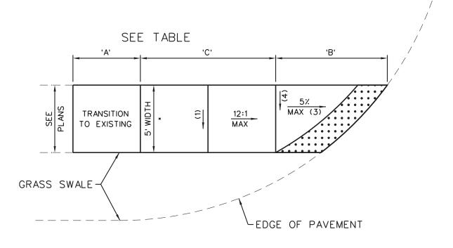
CONFIGURATION S-PERP-4 MOD. TYPE B CURB RAMP SINGLE PERPENDICULAR, LARGE RADIUS, GRASS BUFFER
