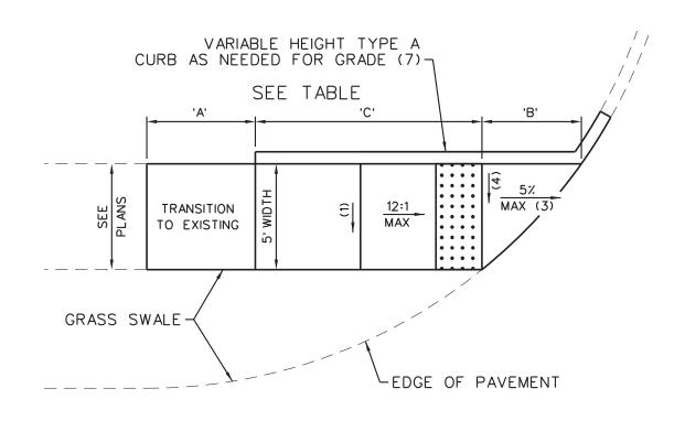
CONFIGURATION S-PERP-3 MOD. TYPE B CURB RAMP SINGLE PERPENDICULAR, SMALL RADIUS, GRASS BUFFER
