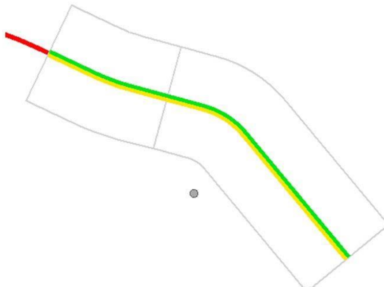
Two lanes defined, yellow and green; one each side of baseline reference (red)
