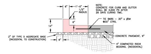
CONCRETE CURB AND GUTTER
