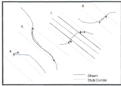
that a culvert will be placed relatively perpendicular to the roadway, thereby reducing the length of stream channel. The same method was used to measure the stream on each side of the existing alignment between corridor lines when the alternative was on existing alignment (c). This type of impact was described as a culvert extension. Example (d) demonstrates how a simple stream crossing was measured and assumed that the culvert would be at the
