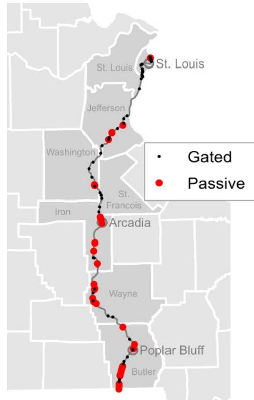
Figure 3 maps the relevant railroad and subdivision for each highway-rail grade crossing along the corridor. The majority of the corridor – 83 public highway-rail grade crossings – is on UP tracks; the remaining 15 crossings are on tracks owned by the TRRA.
