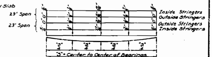
HALF SECTION THROUGH SPANS REQUIRING 14", 16" & 18" STRINGERS
