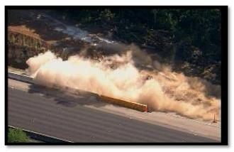
minimize workzone spaces to maintain full I-270 capacity. The use of impact attenuators in the form of jersey barrier design was implemented to allow for crash cushions that took up less space than the typical trashcan styles.
