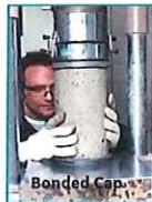
Bonded Cap Sulfur mortar cap AASHTO T231
