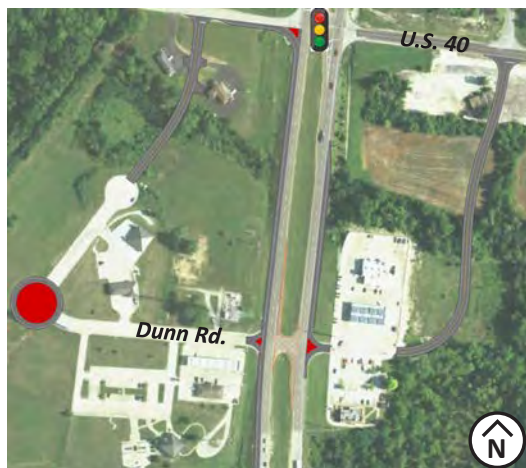
Option #1: Right-in/Right-out at Dunn Rd. and construct west & east backage roads
