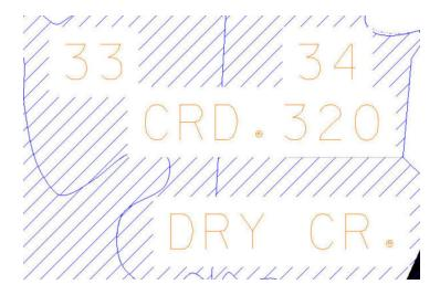
Multi-line text placed with masking and no border
