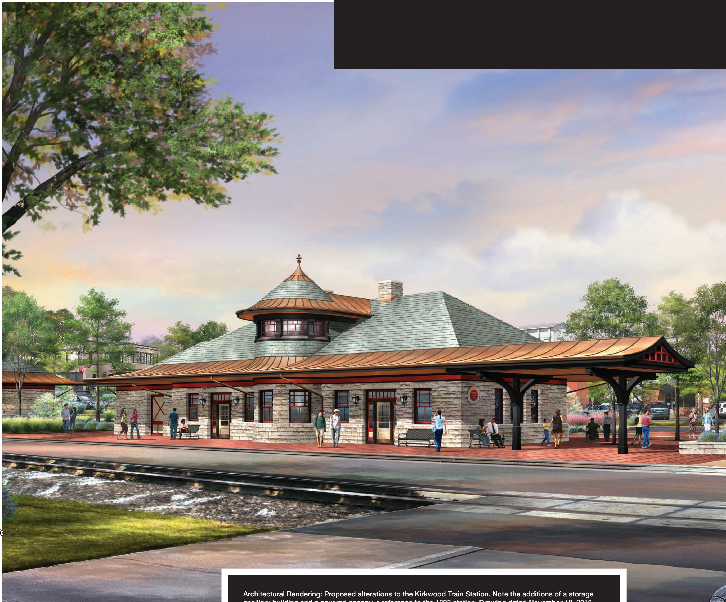
Architectural Rendering: Proposed alterations to the Kirkwood Train Station. Note the additions of a storage ancillary building and a covered canopy, a reference to the 1893 station. Drawing dated November 10, 2016. Photo credit: Dickinson Hussman Architects
