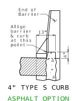
ALTERNATE DETAILS FOR TYPE B BARRIER (SBC)
